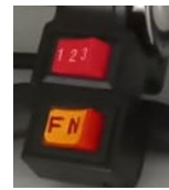
Figure 10 BLE Cluster: Gear, Neutral / Forward buttons
