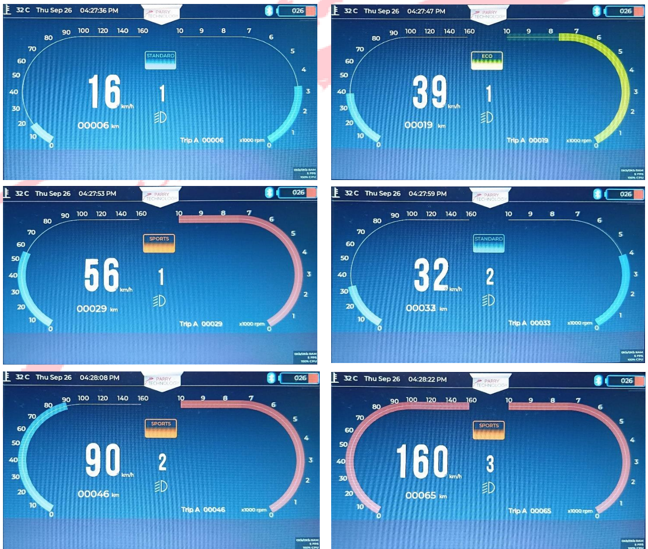
Figure 12 Cluster HMI: Speed / RPM, Gear Position, Speed Mode snapshots
