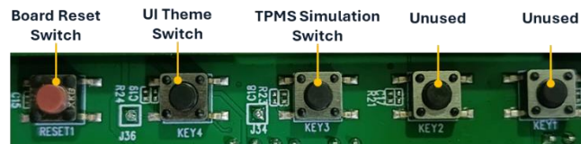
Figure 7 BLE Cluster: Button controls
