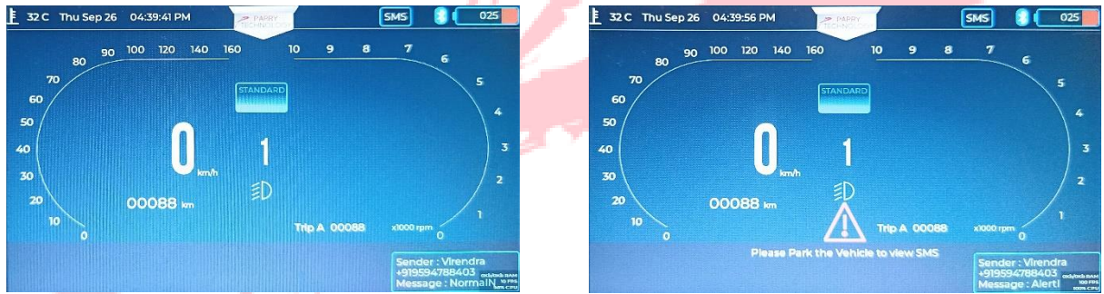
Figure 18 Cluster HMI: SMS Notification (Normal / ALERT)
