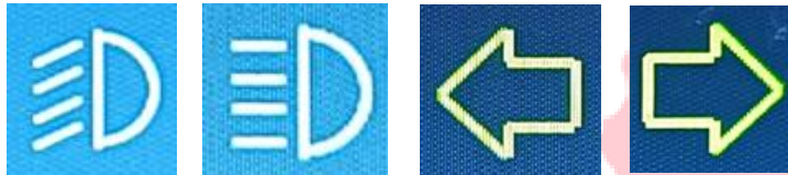
Figure 13 Cluster HMI: High Beam / Low Beam, Indicator elements snapshots
