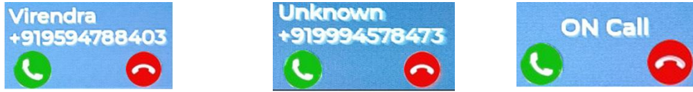
Figure 17 Cluster HMI: Incoming Call Notification and Active Call notification
