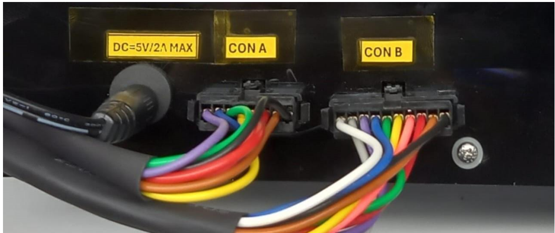
Figure 4 BLE Cluster – Connection with Cluster enclosure and handle-bar assembly
